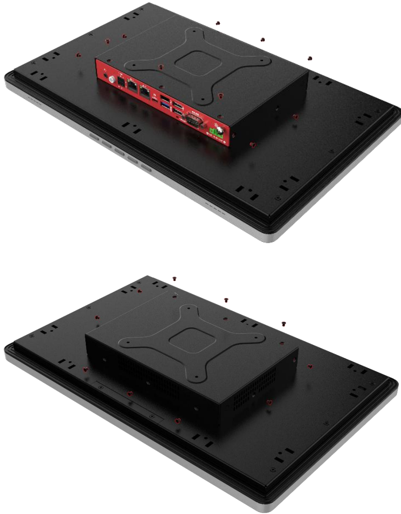
Figure 3-1: AURA-xxx-RK3576 Series Back Cover Retention Screws
